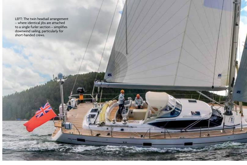
the windward jib. The accumulated wind is redirected into the leeward jib which would otherwise be blanketed by the mainsail. To gybe, simply haul and release the mainsheet onto the new tack leaving the whisker poles and jib sheets unaltered.
